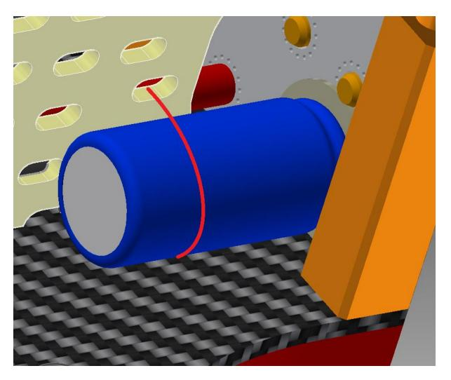
Solder the leads on the rear side (XT60 side) of the pdb firmly before trimming the leads. As the pads are small, we suggest a decent size 'lump' of solder.
