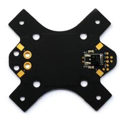
The Kraken PDB 1.0 is made finished with high quality matt black and gold pads. They PCB material is ROHS compliant.
